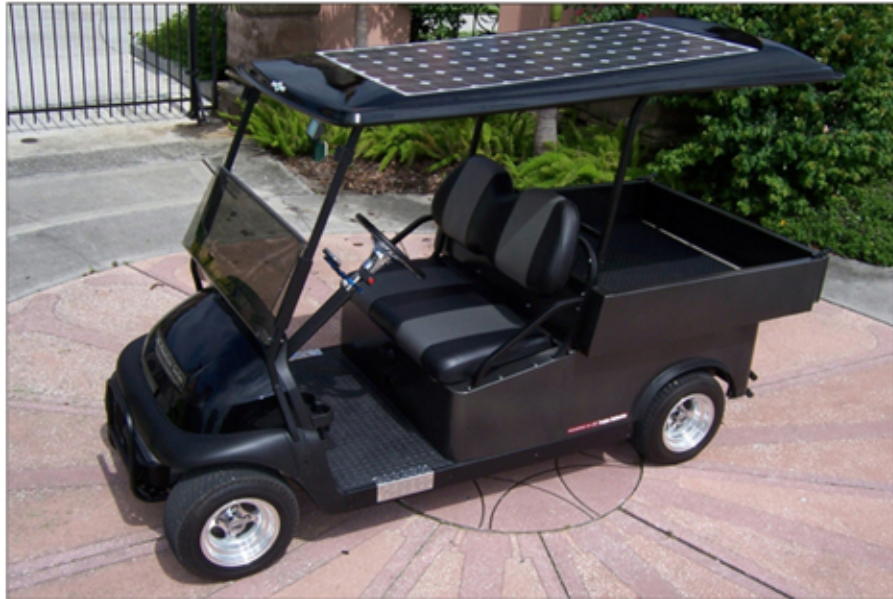
The solar panel allows up to 10 miles of travel. (Photo: Courtesy of Cruise Car, Inc.)
